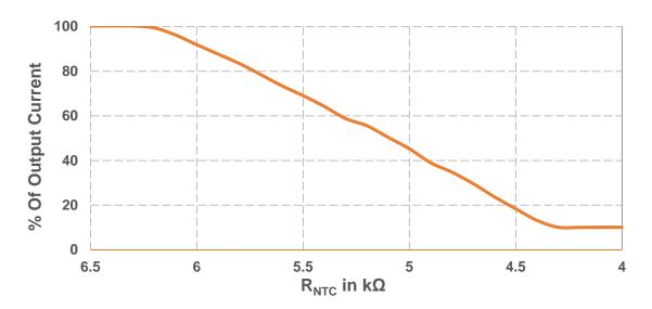
Derating start =  $6.3k\Omega$ ; Derating end =  $4.3k\Omega$ ; Min output level = 10%
