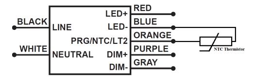
In the end application, care must be taken to place the NTC thermistor close to the hottest spot on the LED module. If LED thermal protection is not required the NTC port on the LED power supply connector can be left open. Vishay, EPCOS, Murata, Panasonic are some of the manufacturers of NTC thermistor. EPCOS part number for reference only **B57164K153J** ( $15k\Omega$  @  $25^{\circ}$ C). Murata part number for reference only - **NCP03XH223J05RL** ( $22k\Omega$  @  $25^{\circ}$ C)
