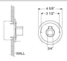
CAST BACK PLATE MOUNTING DETAIL
