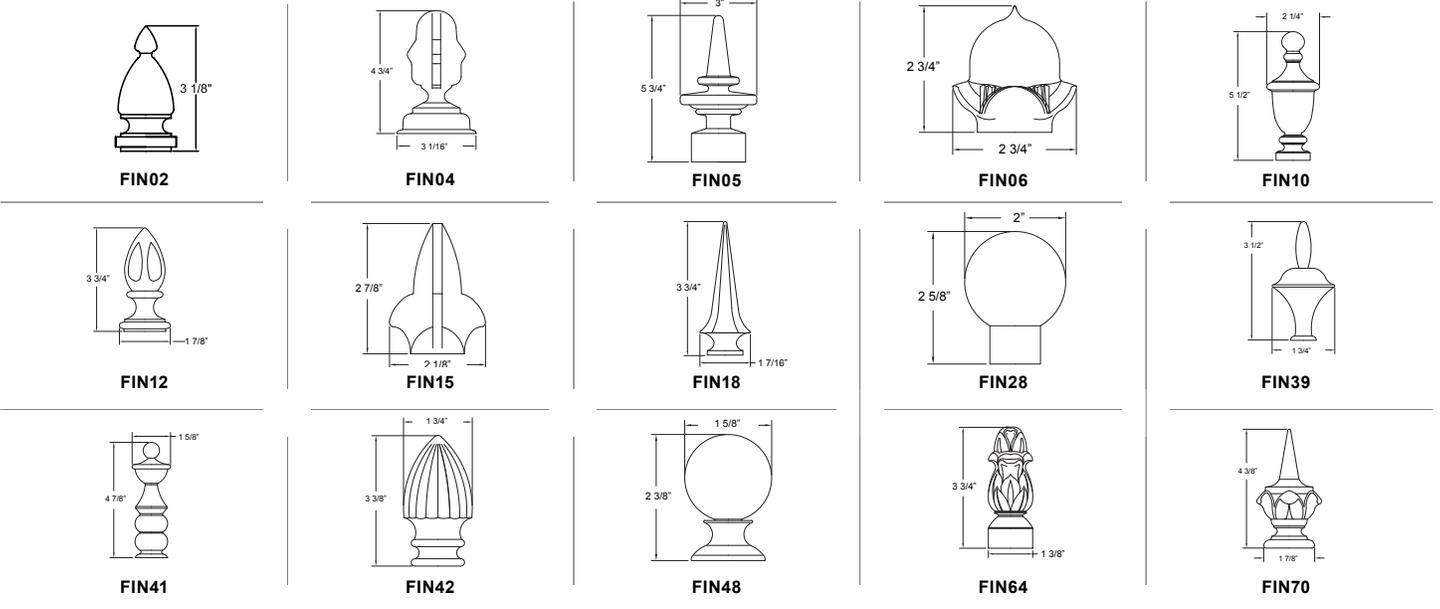
**POST MOUNTS** - See Post Arm Section on Website for Specification Sheets and additional post arms. Dimensions are Projection x Height
